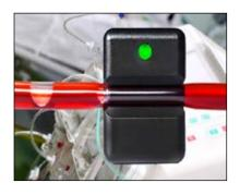
AD8/AD9 non-invasive air bubble & air-in-line sensors incorporate the latest ultrasonic technology. Introtek AD8 (for rigid tubing) and AD9 (for soft tubing) sensors incorporate the latest generation of pulse-type ultrasonic circuitry. Integral to the sensor's assembly, the Micro-Electronic Controller (MEC) features programmable algorithms for functionality control. Response times, time delays and other functions are programmable to specific requirements.
